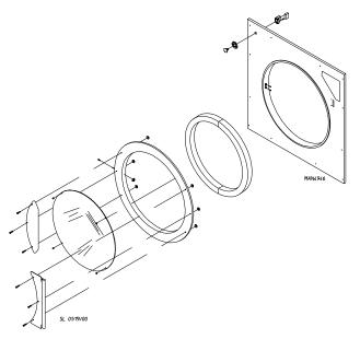
**IMPORTANT:** Do not press hard or silicone thickness between the glass and door will be reduced, resulting in poor bonding.
